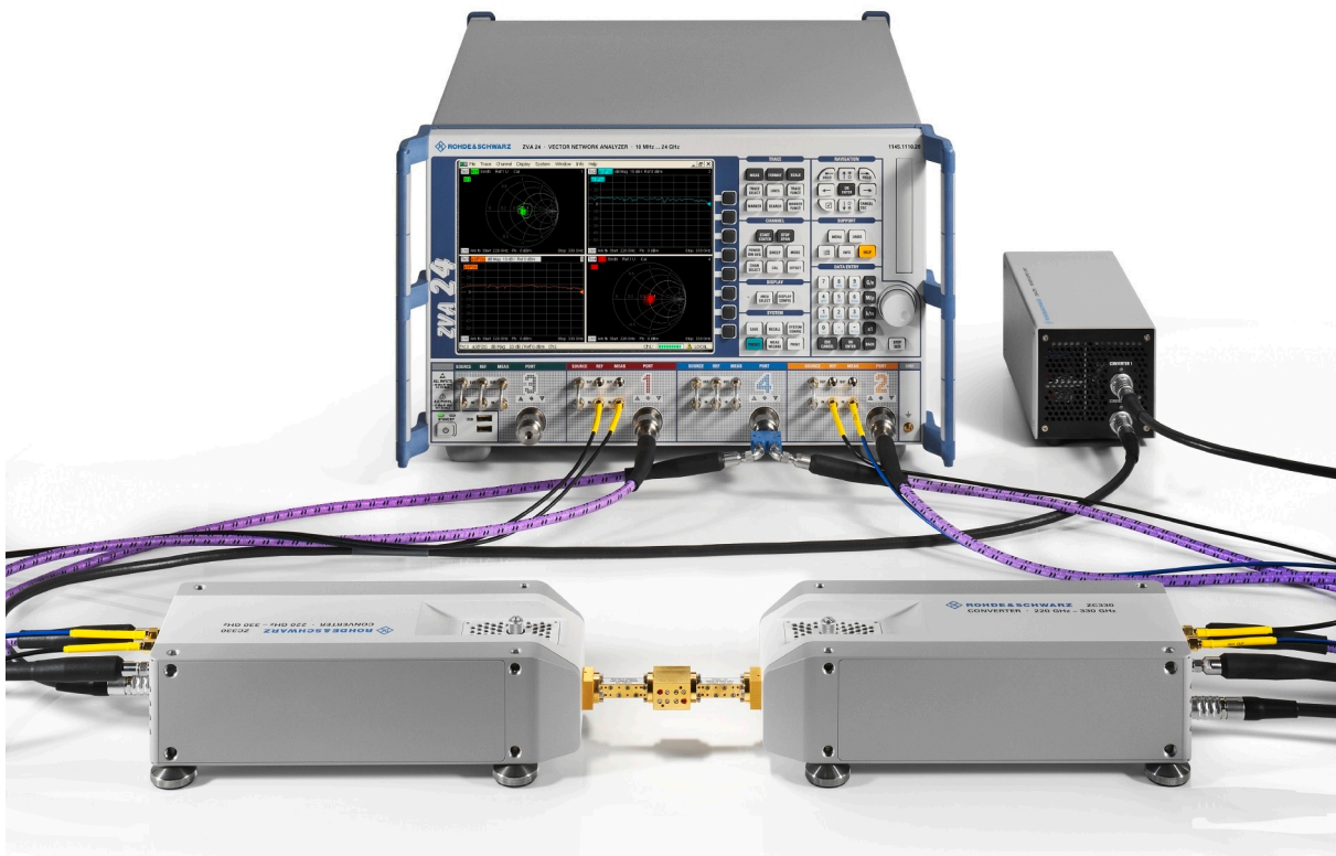
Fig. 2-5: Test setup for 2-port transmission measurement with R&S ZC330 and a NWA with four sources
